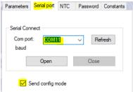
The Com Port for the configurator may have a different number, com9, com7 etc. "Send config mode" should be checked by default. Please check this box if this is not the case.
