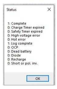
Complete: Yes. This means that the charger completed the charge cycle. Battery is full and the charger completed the charge cycle.
