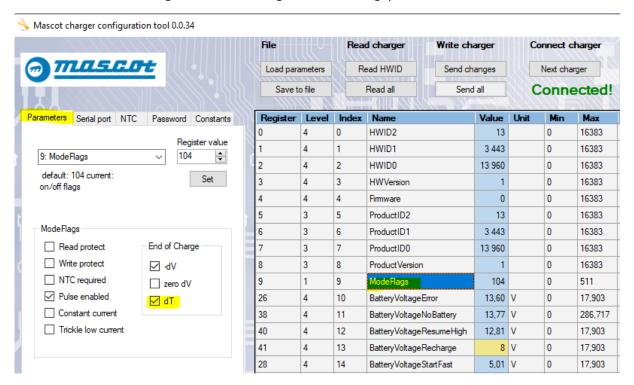
As you can see in the mode flag section the dT checkbox is checked and thereby enabled. The same is -dV detection. These are the EoC methods recommended by Mascot. Mascot do not recommend using Zero dV because this may cause premature EoC detection. Please contact Mascot if you want to fine tune Zero dV parameters.
