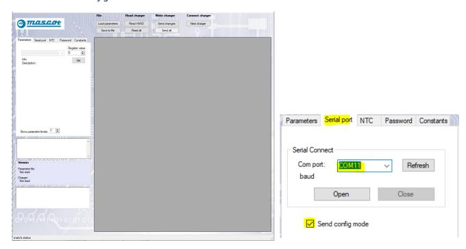
Go to the serial port tab and select the correct Com port. Click Refresh if the port is not listed:
