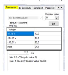
To change the -dV level simply change the value in the matrix in the voltage range applicable.
